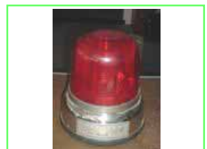
Light, "Strobe Commander" Red Rooftop Light
